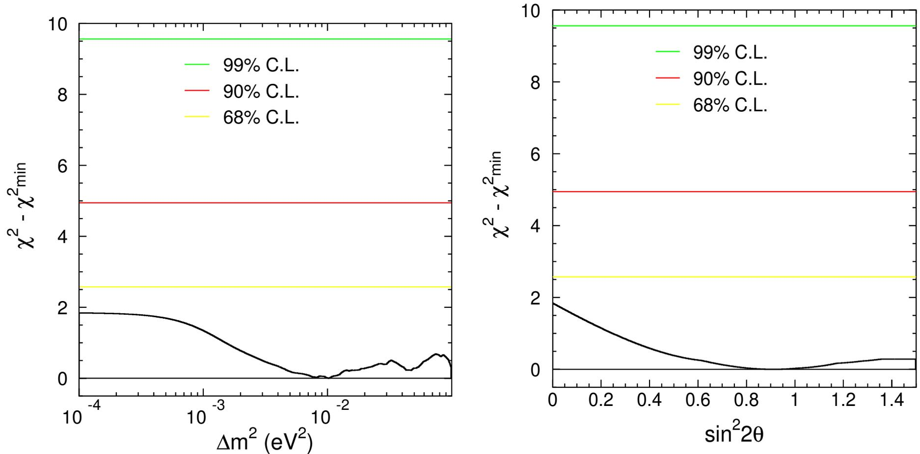
Null oscillation allowed even at 68 % confidence level as expected for this high energy  $\nu_{\mu}$  with mean energy of  $\sim 1$  TeV
