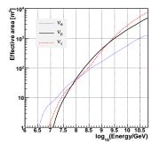
Fig. 3. The effective area for each flavor neutrino after applying the signal selection criteria averaged over all solid angles. Blue dotted line represents  $\nu_e$ , black solid line for  $\nu_\mu$  and red dashed line for  $\nu_\tau$ .
