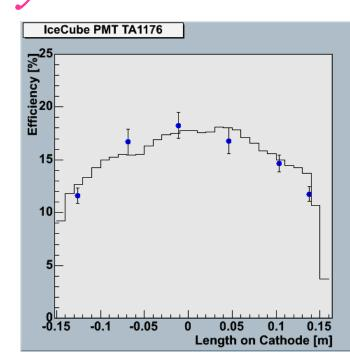
The data points in the left panels show the determined detection efficiency as a function of the distance from the cathode center. The histogram shows the two dimensionally scanned relative collection efficiency described above, after applying the appropriate normalization.
