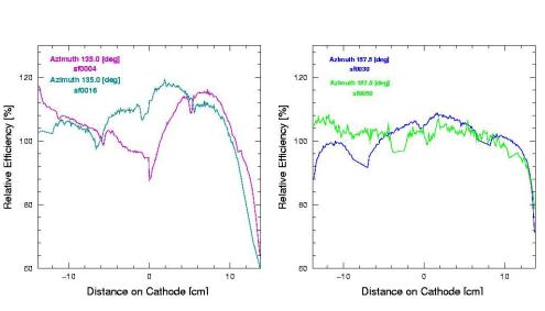
The collection efficiency depends on where a photoelectron is emitted on the photo-cathod surface. The figure below shows our scan results of 8 IceCube PMTs.
